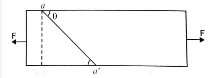
Consider a plane making an angle  $\theta$  with the length. What are the tensile and shering stresses on this plane? (a) For what angle is the tensile stress a maximum? (b) For what angle is the shearing stress a maximum?
