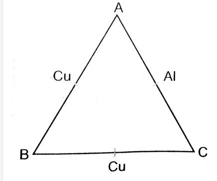
it is heated in such a way that temperature of each rod increases by  $\Delta T$ . Find change in the angle ABC. [Coeff. Of linear expansion for Cu. is  $\alpha_1$ , Coeff. of linear expansion for Al is  $\alpha_2$ ]
