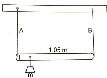
A. Mass m should by suspended close to wire A to have equal stresses in both the wires
