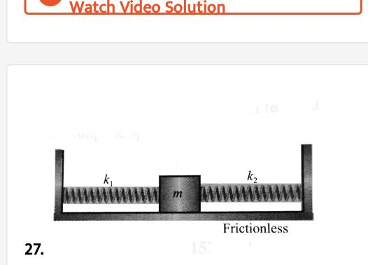
Two springs with negligible masses and force constants  $k_1 = 200 \frac{N}{m}$  and  $K_2 = 160 \frac{N}{m}$  are attached to the block of mass m = 10kg as shown in the fig. Initially the block is at rest, at the equilibrium position which both springs are neither stretched nor compressed. At time t = 0, sharp impulse of 50Ns is given to the block with a hammer along the spring.
