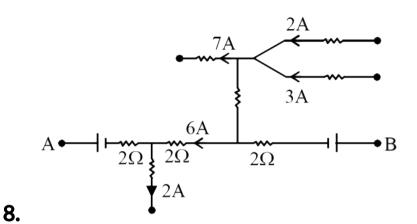
In the above circuit diagram emf of two batteries are equal , then the potential difference  $V_A\!-V_B$  between terminals A and B will be
