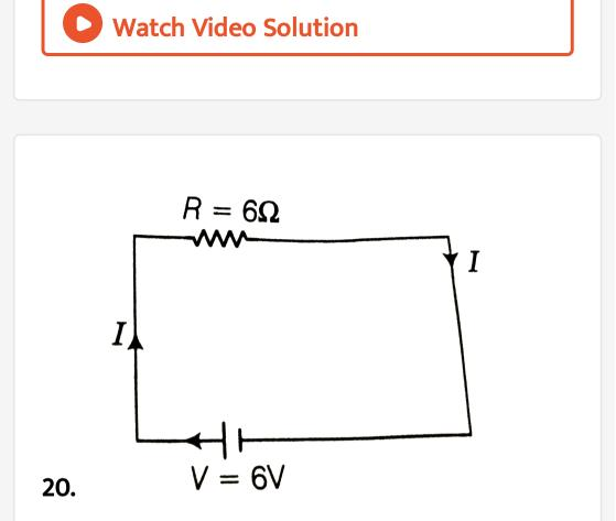
(a). Consider circuit in figure. How much energy is absorbed by electrons from the initial state of no current (ignore thermal motion) to the state of drift velocity?
