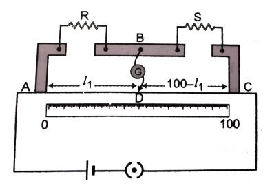
A. The meter bridge can have no other neutral. A point for this set of resistances
