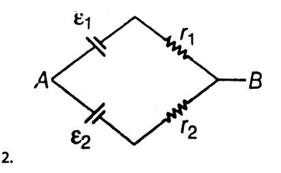
Two batteries of emf  $\varepsilon_1$  and  $\varepsilon_2(\varepsilon_2 > \varepsilon_1)$  and internal resistance  $r_1$  and  $r_2$  respectively are connected in parallel as shown in figure.
