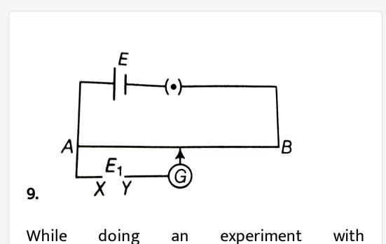
potentiometer (figure) it was found that the deflection is one sided and (i) the deflection decreased while moving from one and A of the wire, to the end R, (ii) the deflection increased, while the jockey was moved towards the end D. (i). Which terminal positive or negative of the cell  $E_1$  is connected at X in case (i) and how is  $E_1$ , related to E? (ii). Which terminal of the cell  $E_1$  is connected at X in case (1 in 1)?
