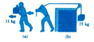
**8.** In figure (i) the man walks 2 m carrying a mass of 15 kg on his hands .In figure (ii), he walks the same distance pulling the rope behind him. The rope goes over a pulley, and a mass of 15 kg hangs at its other end. In which case is the work done greater?
