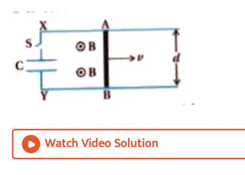
**9.** Find the current in the sliding rod AB (resistance = R) for the arrangement shown in figure.  $\overrightarrow{B}$  is constant and is out of the paper. Parallel wires have no resistance, v is constant. Switch S is closed at time t = 0.
