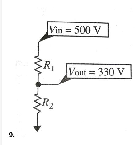
A voltage is a simple circuit that converts a large voltage into a smaller one. The figure
