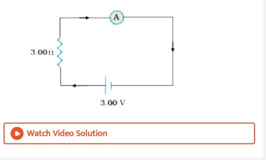
22. In the circuit the current is to be measured. What is the value of the current if the ammeter shown (a) is a galvanometer with a resistance  $R_G = 60.00\Omega$ , (b) is a galvanometer described in (a) but converted to an ammeter by a shunt resistance  $r_s=0.02\Omega$ , (c ) is
