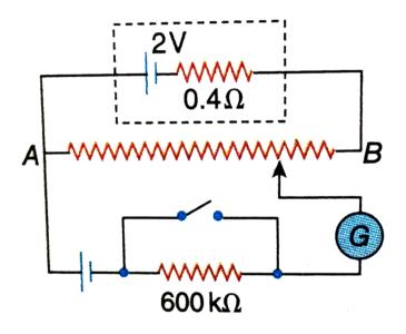
Would the circuit work well for determining an extremely small emf , say of the order of a few m V? If not , how will you modify the circuit ?
