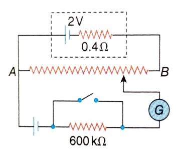
Would the method work in the above situation of the drive cell of the potentiometer had an emf of 1.0 V instead of 2.0 V?
