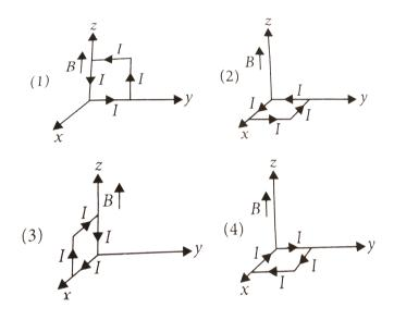
If there is a uniform magnetic field of 0.3 T in the positive z-direction, in which orientations the loop would be in (i) stable equilibrium and (ii) unstable equilibrium.
