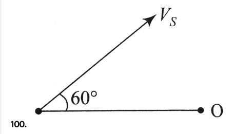
A source of sound S emitting waves of frequency 100Hz and an observer O are located at some distance from each other. The source is moving with a speed of  $19.4ms^{-1}$  at an angle of  $60^\circ$  with the source observer line as shown in the figure. The observer is at rest. The apparent frequency observed by the observer (velocity of sound in air  $330ms^{-1}$ ) is
