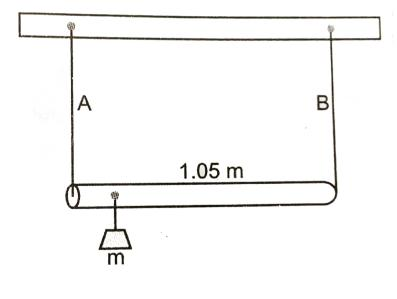
**19.** A mild steel wire of length 1.0 m and cross-sectional are  $0.5 \times 10^{-20} cm^2$  is streached, well within its elastic limit, horizontally between two pillars. A mass of 100 g is suspended from the mid point of the wire, calculate the depression at the mid point.
