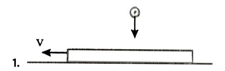
A board is moving with velocity v on а smoother horizontal plane. The upper surface of the board is rough on which a ball falls with velocity v and rebounds with velocity  $\frac{v}{2}$ . The mass of the board is same as that of ball. After the collision. the board comes to state of rest. The co-efficient of friction between the board and the ball is
