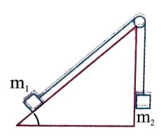
A. If  $m_1=m_2$ , the mass  $m_1$  first begin to move up inclined plane when the angle of inclination heta, then  $\mu=\sec heta- an heta$
