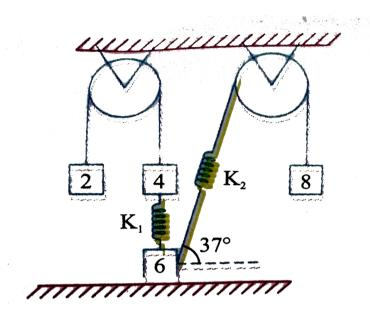
A. Minimum coefficent of friction required between 6kg block and ground  $\mu=2$  such that system is in equilibrium.
