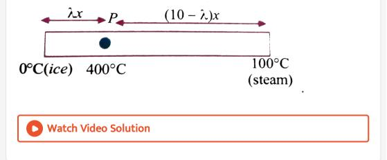
**6.** Find the value of the thermal resistance of the non-uniform cylindrical rod of thermal conductivity K and length I as shown in
