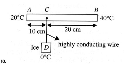
As shown in Fig. AB is rod of length 30 cm and area of cross section 1.0  $cm^2$  and thermal conductivity 336 SI units. The ends A and B are maintained at temperatures  $20^{\circ}C$  and  $40^{\circ}C$ , respectively .A point C of this rod is connected to a box D, containing ice at  $0^{\circ}C$  through a highly conducting wire of negligible heat capacity. The rate at which ice melts in the box is (assume latent heat of fusion for ice  $L_f = 80cal/g$ )
