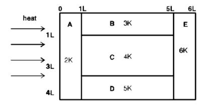
A. heat flow through A and E slabs are same
