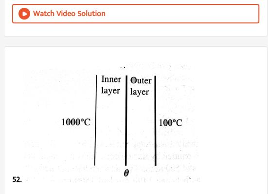
The temperature drop through a two layer furnace wall is  $900^{\circ}C$ . Each layer is of equal area of cross section. Which of the following actions will result in lowering the temperature  $\theta$  of the interface?
