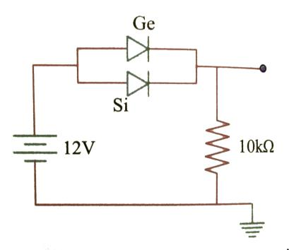
**9.** Find the maximum voltage across AB in the circuit shown in Fig. Assume that diode is ideal.
