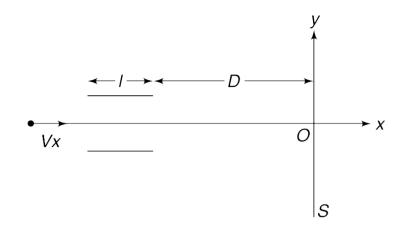
(c) Now the field region is filled with a uniform electric (E) and magnetic field (B) both directed in positive y direction. A beam of protons and some other positive ion enters the region trav- elling along x direction. The particles hit the screen along two curved paths. Explain. Draw the two curves in yz plane and point out which one represents the protons.
