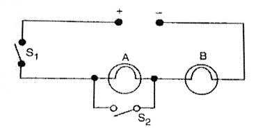
(a) When  $S_1$  and  $S_2$  are closed, lamps A and B are lit.
