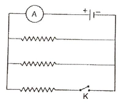
With the switch K open, the ammeter reads 0.6A. What will be the
