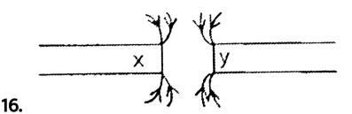
The above diagrame is the pattern of magnetic lines of force obtained when two magnets are placed with their magnetic axes coinciding. The magnetic poles x and y are\_\_\_\_and \_\_respectively.
