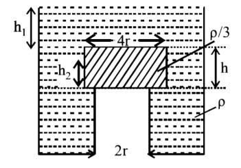
Situation I: Initially, the tank is filled with water of density  $\rho$  to a height such that the height of water above the top of the block is  $h_1$ (measured from the top of the block). Situation II: The water is removed from the tank to a height  $h_2$  (measured from the bottom of the block), as shown in the figure. The height  $h_2$  is smaller than h (height of the
