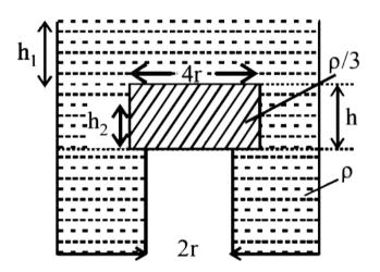
Situation I: Initially, the tank is filled with water of density ho to a height such that the height of water above the top of the block is  $h_1$  (measured from the top of the block).
