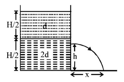
(a) A homogeneous solid cylinder of length L(L < H/2), cross-sectional area A/5 is immersed such that it floats with its axis vertical at the liquid-liquid interface with length L/4 in the denser liquid. Determine: (i) the density D of the solid and (ii) the total pressure at the bottom of the container. (b) The cylinder is removed and the original arrangement is restored. A tiny hole of area s(s < < A) is punched on the vertical side of the container at a height h(h < H/2).
