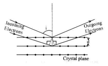
If a strong diffraction peak is observed when electrons are incident at an angle i from the normal to the crystal planes with distance d between them (see fig) de Brogle wavelength  $\lambda_{dB}$  of electrons can be calculated by the relationship (n is an intenger)
