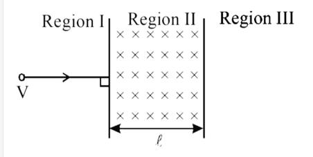
A. The particle enters Region III only if its velocity  $v < \frac{qlB}{m}$ B. The particle enters Region III only if its velocity  $v > \frac{qlB}{m}$
