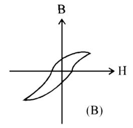
These materials are used to make magnets for electric generators, transformer core and electromagnet core. Then it is proper to use:
