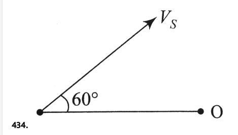
A source of sound *S* emitting waves of frequency 100Hz and an observer *O* are located at some distance from each other. The source is moving with a speed of  $19.4ms^{-1}$  at an angle of 60 ° with the source observer line as shown in the figure. The observer is at rest. The apparent frequency observed by the observer (velocity of sound in air  $330ms^{-1}$ ) is
