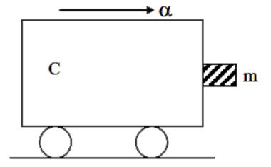
The coefficient of static friction between the block and the cart is  $\mu$ , The accelertion  $\alpha$  of the cart that will prevent the block from failing satisfies -
