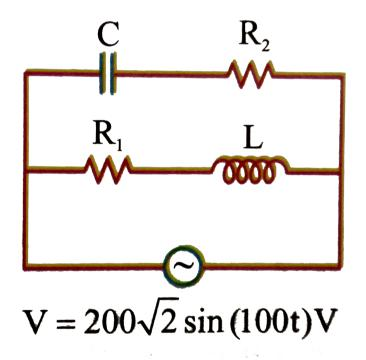
At some instant current in  $L-R_1$  circuit is 10A. At the same instant current in  $C-R_2$  branch will be
