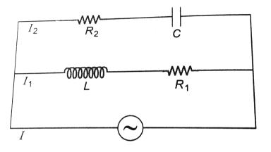
$R_1 = 30\Omega, R_2 = 40\Omega, L = 0.4H$  and  $C = \frac{1}{3}mF$ . Find seven function of time  $I, I_1, I_2, V_{R_1}, V_L, V_{R_2}$  and  $V_C$ . Also total power consumed in the circuit. In the given potential function V is in volts and omega in rad/s.
