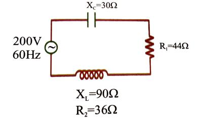
The power dissipated in the inductance coil is
