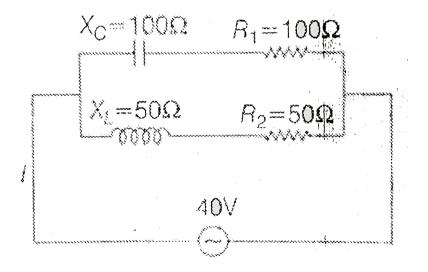
A. The voltage across  $100\Omega$  resistor  $20\sqrt{2}V$
