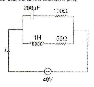
A. The voltage across  $100\Omega$  resistor  $20\sqrt{2}V$
