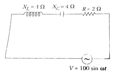
A. The rms value of current through the circuit is  $i_{rms}$  =  $5\sqrt{2}$  A
