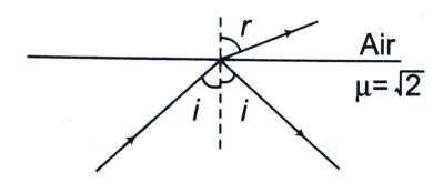
In the figure, i is increased from  $0^{\circ}$  to  $90^{\circ}$  . But ray of light is travelling from denser to rarer medium. Therefore, TIR will take place when  $i>\theta_C$ ,
