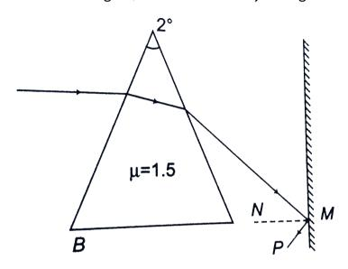
ray of light retraces its path after reflection from M ray of light MP turns in the direction of MN.
