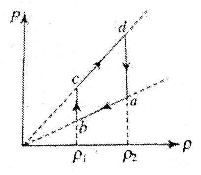
A. Work done by the gas in the process 'bc' is zero
