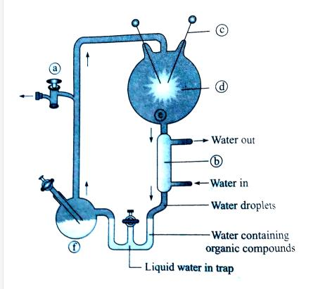
A. a- condenser, b- to vaccum pump, c - electrode, d- spark discharge, e
