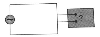
Measurements, outside the box reveals that  $e=75\sin(\omega t)$  volts,  $i=1.5\sin(\omega t+45^\circ)$
