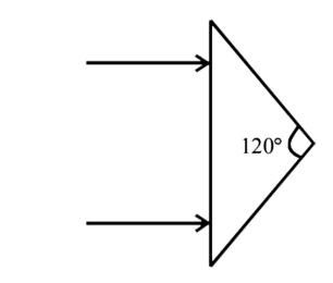
An isosceles prism of angle 120degree has a refractive index 1.44. Two parallel monochromatic rays enter the prism parallel to each other in air as shown. The rays emerge from the opposite faces
