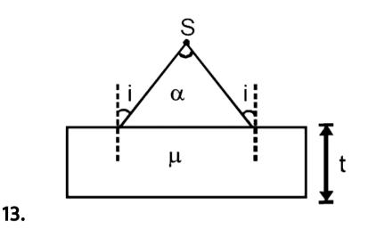
A diverging beam of light from a point source S having divergence angle  $\alpha$ , falls symmetrically on a glass slab as shown. The angles of incidence of the two extreme rays are equal. If the thickness of the glass slab is t and the refractive index n, then the divergence angle of the emergent beam is
