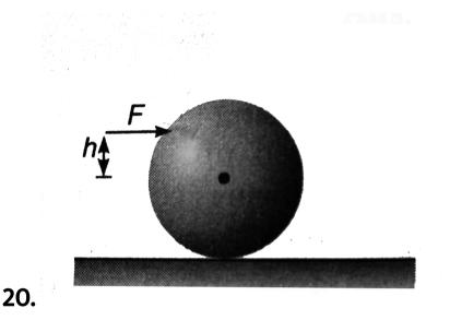
A billiard ball, initially at rest, is given a sharp impulse by a cue. The cue is held horizontally a distance h above the centre line as shown in figure. The ball leaves the cue with a speed  $v_0$ and because of its backward slipping eventually acquires a final
