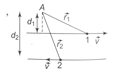
A. Angular momentum  $\overrightarrow{L_1}$  of particle 1 about A is  $\overrightarrow{L_1} = mv(d_1)$   $\odot$ B. Angular momentum  $\overrightarrow{L_2}$  of particle 2 about A is  $\overrightarrow{L_1} = mvr_2$   $\odot$  C. Total angular momentum of the system
