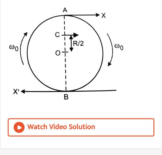
**8.** (i) Explain why friction is necessary to make the disc to roll in the direction indicated. (ii) Give the direction of frictional force at B, and the sense of frictional torque, before perfect
