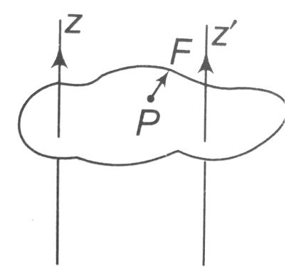
A. Torque  $\tau$  caused by F about z-axis is along - $\hat{k}$ B. Torque au' caused by F about z' axis is along  $\hat{k}$ . C. Torque au caused by F about z-axis is greater in magnitude than that about zaxis.
