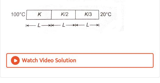
**14.** In the following situations, the length and area of cross-section of each rod is same. Find temperature  $\theta$  at junction of rods.
