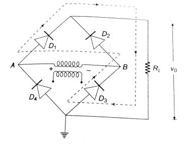
A. when A is positive, B is negative, diodes  $D_1$  and  $D_3$  conducts, the conduction path is shown by dotted lines B. During next half-cycle, diodes  $D_2$  and  $D_4$
