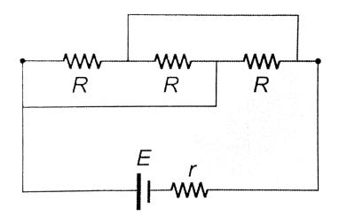
(c) A battery of internal resistance  $4\Omega$  is connected to the network of resistance as shown in the figure. What must be the value of R so that maximum power is delivered to the network? What is that maximum power?
