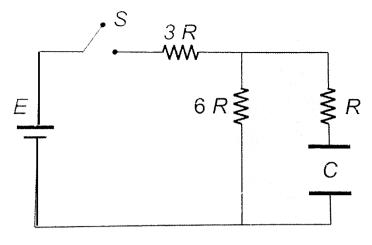
Find (a) equivalent time constant, (b) charge on capacitor in terms of time t.
