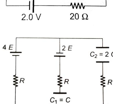
(i) Find ratio of energy stored in capacitors,  $C_1$  and  $(C_2)$
