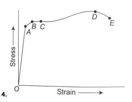
The stress strain graph for a metal wire is as shown in the figure. In the graph, the region in which
