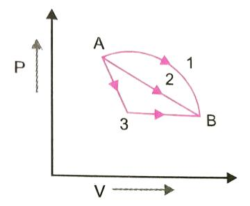
If  $Q_2, Q_3$  indicates the heat absorbed by the gas along the three processes and  $\Delta U_1, \Delta U_2, \Delta U_3$  indicates the change in internal energy along the three processes respectively, then
