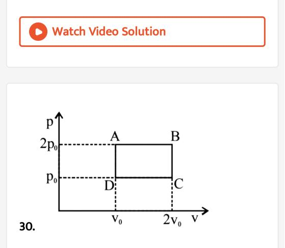
The above p-v diagram represents the thermodynamic cycle of an engine, operating with an ideal monoatomic gas. The amount of heat, extracted from the source in a single cycle is
