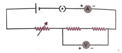
A. Position of voltmeter is incorrect
