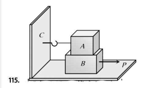
Block A weighing 100 kg rests on a block B and is tied with a horizontal string to the wall at C. Block B weighs 200 kg. The coefficient of friction between A and B is 0.25 and between B and the surface is 1/3. The horizontal force P necessary to move the block B should be  $(g=10m/s^2)$
