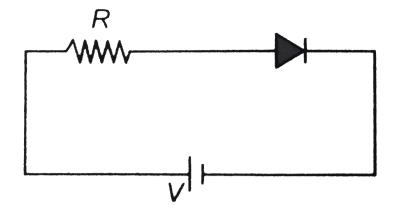
A. In forward biasing the voltage across R is V
