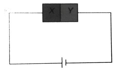
A. X is P -type, Y is N -type and the junction is forward biased
