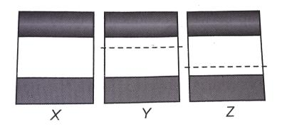
A. Sample X is undoped while samples Y and Z have been doped with a third group and a fifth group impurity respectively
