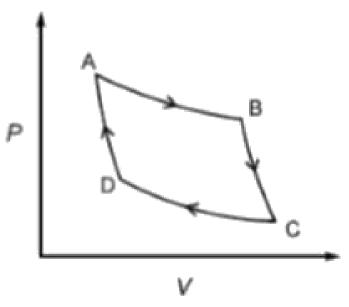
AB and CD are isothermal processes while BC and DA are adiabatic processes. The same cycle in the temperature (T) - entropy (S) plane is :
