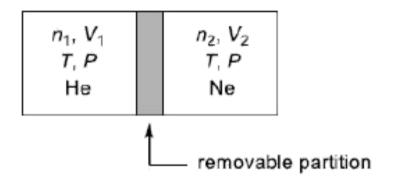
In the first compartment  $n_1$  moles of ideal gas He is present in a volume  $V_1$ . In the second compartment,  $n_2$  moles of ideal gas Ne is present in a volume  $V_2$ . The temperature and pressure in both the compartments are T and P repectively. Assuming R is the gas constant. the total change is entropy upon removing the partition when the gases mix irreversibly is :
