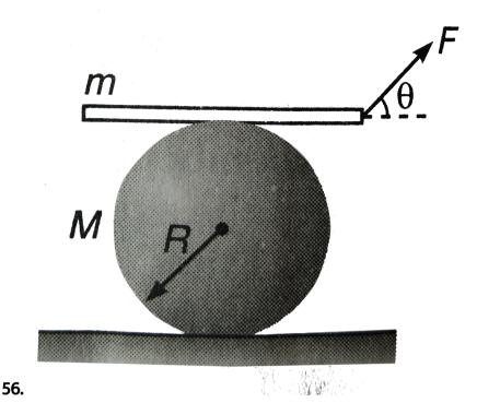
Consider a cylinder of mass M and radius R lying on a rough horizontal plane. It has a plank lying on its top as shown in figure. A force F is applied on the plank such that the plank moves and causes the cylinder to roll the plank always remains horizontal. there is no slipping at any point of contact. Calculate the acceleration of the cylinder and the frictional forces at the two contact.
