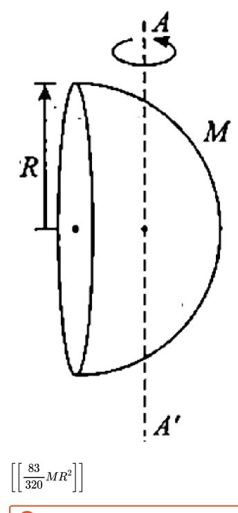
5. Find the of inertia of the half cylinder of mass M shown in figure -
