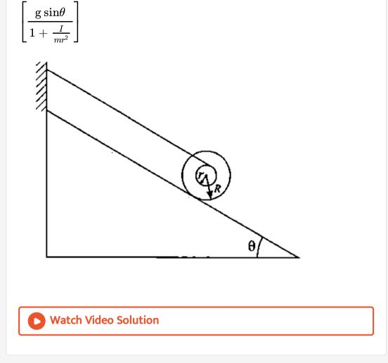
**21.** A uniform solid cylinder of mass M and radius R rolls a rough inclined plane with its axis perpendicular to the line of greatest slope as shown in figure-5.75. As the cylinder rolls it winds up a light string which passes over a light and smooth pulley and attached to a mass m, the part of the string between pulley and cylinder being parallel to
