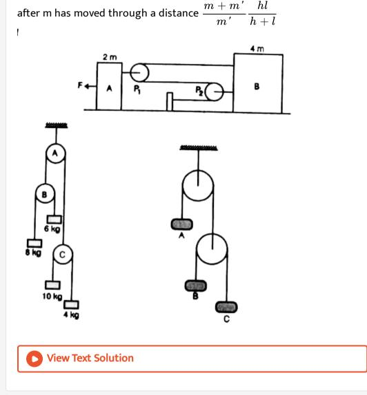
15. Calculate the accelerations of the pulleys B and C and the tension in
