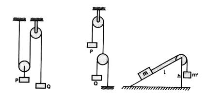
**13.** Neglecting friction and the mass of the pulleys, find the acceleration of the mass Q assuming that P=Q (Figure 5.20).
