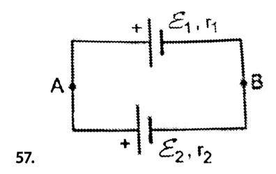
Two cells of unequal emfs,  $\mathcal{E}_1$  and  $\mathcal{E}_2$  and internal resistances  $r_1$  and  $r_2$  are joined as shown.  $V_A$  and  $V_B$  are the potentials at A and B respectively.
