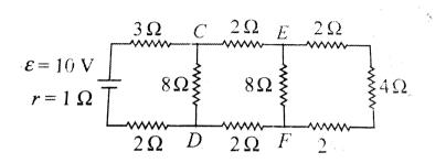
A. The current through the  $3-\Omega s$  resistor is 1A.
