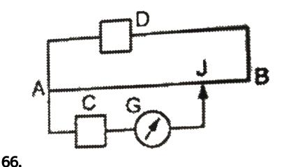
The figure shows a potentiometer arrangement. D is the driving cell. C is the cell whose emf is to be determined. AB is the
