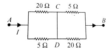
A. The equivalent resistance between A and B is  $8\Omega$
