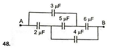
In the circuit shown, the equivalent capacitance between the points A and B is
