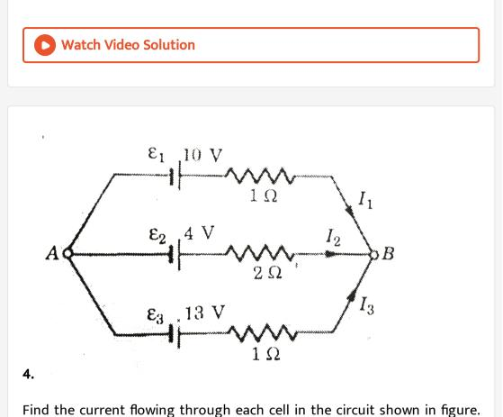
Also calculate the potential difference across the terminals of each cell.
