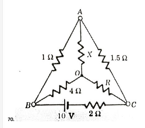
for the network shown in figure, determine the value of R and the current
