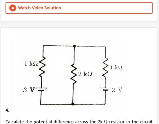
shown in figure. The internal resistance of the cells are negligible.
