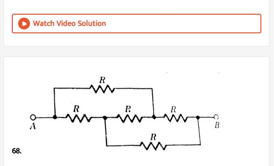
Calculate the equivalent resistance between the points A and B of the network shown in figure.
