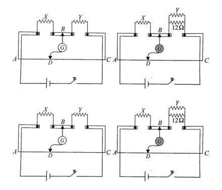
with the help of a movable contact d, one can change the ratio of resistance of the two segments of the wire until a sensitive galvanometer G connected across b and D shows no deflection. The null point is found to be at a distance of 33.7cm. The resistor Y is shunted by a resistance of
