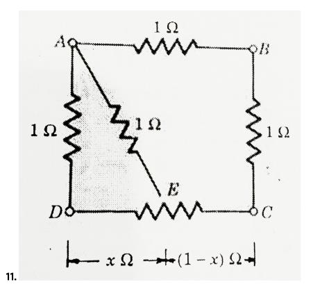
In figure. ABCD is a square where side is a uniform wire of resistance  $1\Omega$ . Find the a point E on CD such that if a uniform wire of resistance  $1\Omega$  is connected across AE and a constant potential difference is applied across A and C the points B and E are equipotential.
