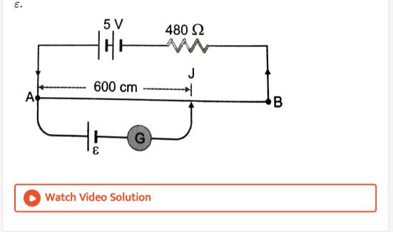
**19.** AB is 1 meter long uniform wire of  $10\Omega$  resistance. Other data are shown in the diagram. Calculate (i) potential gradient along AB (ii)
