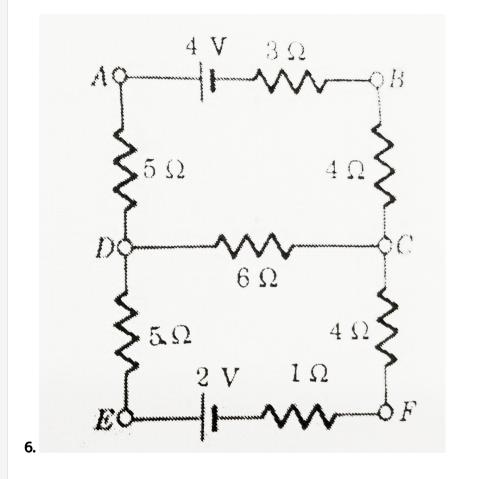
Calculate (i) current in the  $6\Omega$  resistor, (ii) terminal voltage across the 4V
