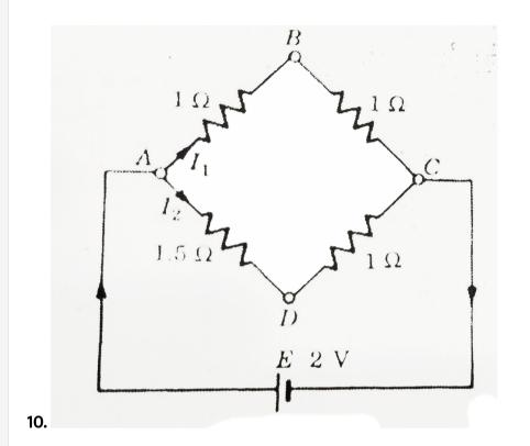
Calculate the potential difference between the junctions B and D in the
