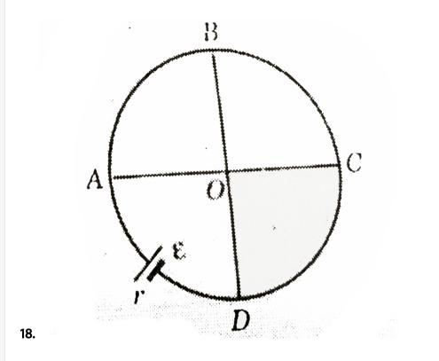
In figure. ABCDA is a uniform circular wire of resistance  $2\Omega$ , AOC and BOD are two wires along two perpendicular diameters of the circle, each having ame resistance  $1\Omega$ . A battery of emf  $\varepsilon$  and internal resistance r is connected between the point A and D. Calculate the equivalent resistance of the network
