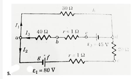
Determine the currents  $I_1$ ,  $I_2$  and  $I_3$  from the network shown in figure.
