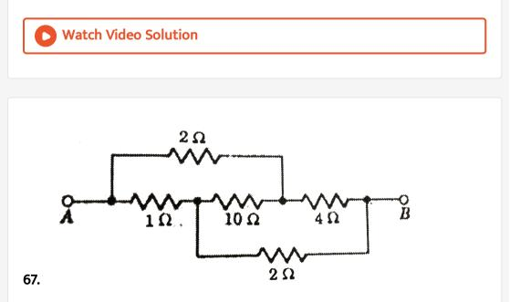
Calculate the equivalent resistance between points A and B of the
