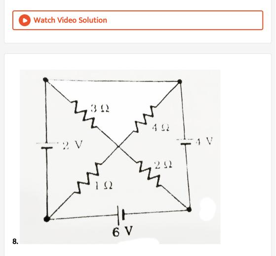
In the network shown in figure. (i) calculate the current of the 6V battery and (ii) determine the potential difference between the points A and B.
