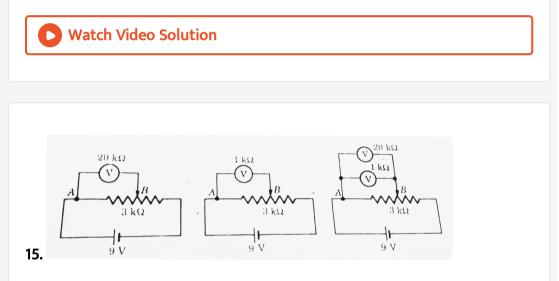
A battery of emf 9 V and negligible internal resistance is connected to a 3 k  $\Omega$  resistor. The potential drop across a part of the resistor (between points A and B in the figure) is measured by (i) a 20 k  $\Omega$  voltmeter, (ii) a 1 k  $\Omega$  voltmeter. in (iii). both the voltmeter are connected across AB. in which case would you get the (a) highest, (b) lowest reading?
