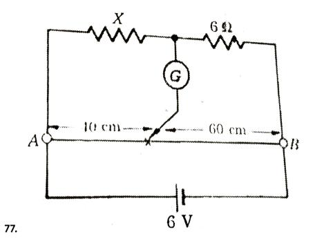
In the circuit shown in figure. A metre bridge is shown in its balanced state. The metre bridge wire has a resistance of a 4 ohm/cm. calculate the value of the unknown resistance X and the current drawn from the battery of negligible resistance.
