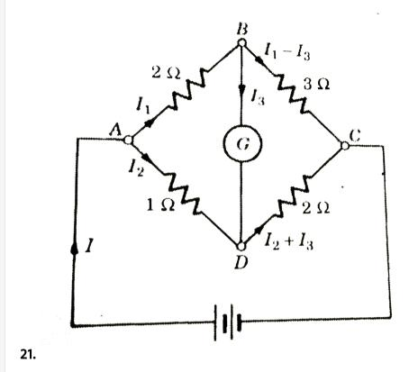
In the circuit shown in figure. Find the currents I,  $I_1$ ,  $I_2$  and  $I_3$  given that emf of th battery=2V, internal resistance of the battery =  $2\Omega$  and resistance of the galvanomter =  $4\Omega$ .
