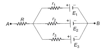
a. Find the potential differece between the points A and B and the currents through each branch.
