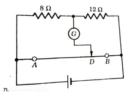
The potentiometer wire AB shown in figure. Is 40 cm long. Where should the free end of the galvanometer be connected on AB so that the galvanometer may show zero deflection?
