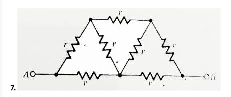
In the network as shown in figure. Each resistance r is of  $2\Omega$  find the effective resistance between points A and B.
