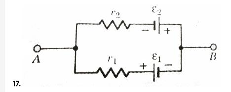
find the emf  $(\varepsilon_0)$  and internal resistance  $(r_0)$  if a battery which is equivalent to a parallel combination of two batteries of emfs  $\varepsilon_1$  and  $\varepsilon_2$ and internal resistances  $r_1$  and  $r_2$  respectively, with polarities as shown in figure.
