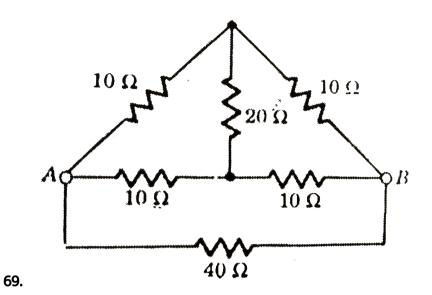
Calculate the resistance between the points A and B of the network shown in figure.
