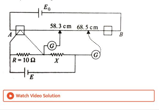
**22.** Figure 6.13 shows a 2.0V potentiometer used for the determination of internal resistance of a 1.5V cell. The balance point of the cell in open circuit is 76.3cm. Whan a resistor of  $9.5\Omega$  is used in the external circuit of
