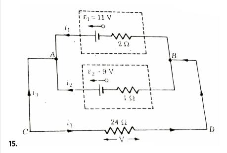
Compute the values of  $i_1$ ,  $i_2$ ,  $i_3$  and V in the circuit, shown in figure. The emf and the internal resistance of the upper cell are 11V and  $2\Omega$ , and of the lower cell are 9 V and  $1\Omega$ .
