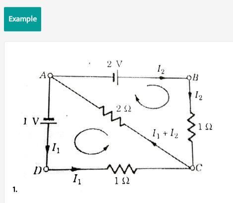
In the circuit shown in figure. Calculate the current in each resistance. The internal resistnaces of the cells are negligible.
