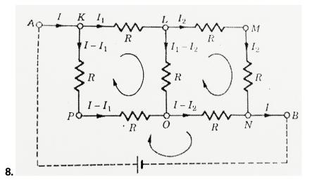
Find the equivalent resistance between the terminals A and B in the network shown figure. Given each resistor R of  $10\Omega$ .
