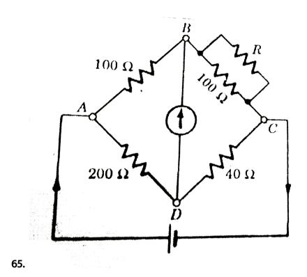
The wheatstone's bridge of figure. Is showing no deflection in the galvanometer joined between the points B and D. compute the value of R.
