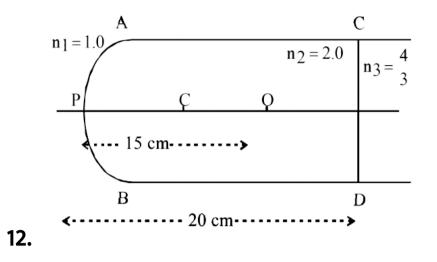
A slab of a material of refractive index 2 shown in fig. has a curved surface APB of radius of curvature 10 cm and a plane surface CD. On the left of APB is air and on the right CD is water with refractive indices as given in the figure. An object O is placed at a distance of 15 cm from the pole P as shown. The distance of the final image of O from P, as viewed from the left is.....
