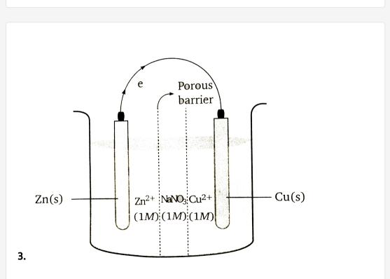
A Galvanic cell consits of three compartment as shown in figure. The first compartment contain  $ZnSO_4$ (1M) and III compartment contain  $CuSO_4$ (1M). The mid compartment contain  $NaNO_3$  (1M). Each compartment contain 1L solution:  $E^{\,\circ}_{Zn^{2+}\,/\,Zn}=~-$  0.76,  $E^{\,\circ}_{Cu^{2+}\,/\,Cu}=~+$  0.34
