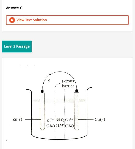
A Galvanic cell consits of three compartment as shown in figure. The first compartment contain  $ZnSO_4$ (1M) and III compartment contain  $CuSO_4$ (1M). The mid compartment contain  $NaNO_3$  (1M). Each compartment contain 1L solution:  $E^{\,\circ}_{Zn^{2+}\,/\,Zn}=~-$  0.76,  $E^{\,\circ}_{Cu^{2+}\,/\,Cu}=~+$  0.34,
