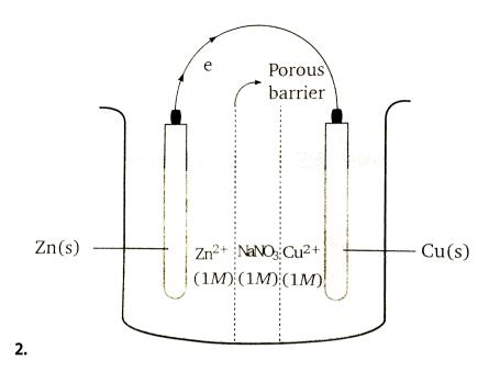
A Galvanic cell consits of three compartment as shown in figure. The first compartment contain  $ZnSO_4$ (1M) and III compartment contain  $CuSO_4$ (1M). The mid compartment contain  $NaNO_3$  (1M). Each compartment contain 1L solution:
