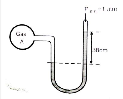
If the same liquid is used in barometer to measure the atmospheric pressure, then what will be the lengh of the liquid columnm which exerts pressure equal to 1 atm ? (density of  $Hg=13.6g/cm^3$ )
