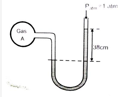
If the same liquid is used in barometer to measure the atmospheric pressure, then what will be the length of the liquid column, which exerts pressure equal to 1 atm ? (density of Hg =  $13.6g/cm^3$ )
