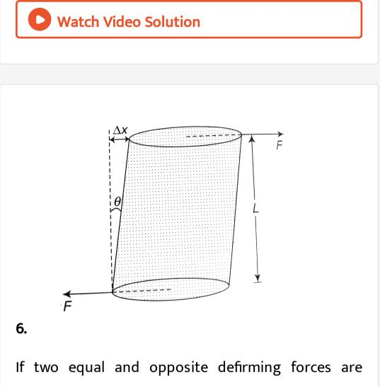
applied parallel to the cross sectional area of the cylinder as shown in the figure, there is a relative displacement between the oppsite faces of the cylinder. The ratio of Ax to L is known as A. loagitudinal strain
