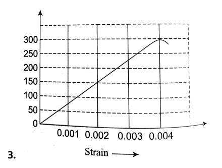
Figure shows the strain stress curve for a given material. The Young's modulus of the material is
