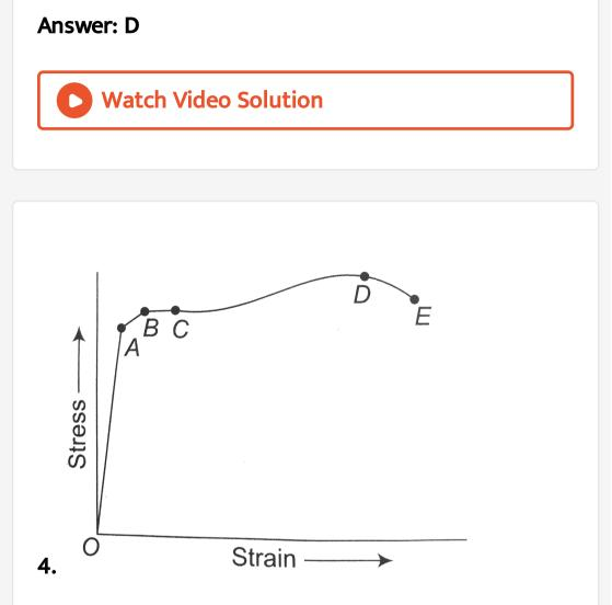
The stress strain graph for a metal wire is as shown in the figure. In the graph, the region in which Hooke's law is obeyed, the ultimate strength and
