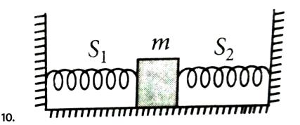
When a mass m is connected individually to two springs  $S_1$  and  $S_2$ , the oscillation frequencies are  $v_1$  and  $v_2$ . If the same mass is attached to the two springs as shown in figure, the oscillation frequency would be
