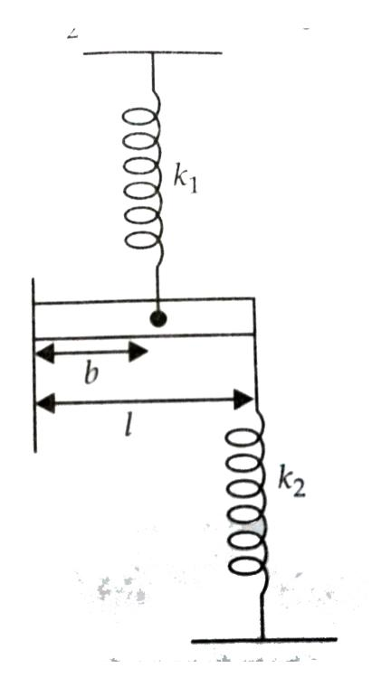
A rod of mass m and length I is connected by two spring of spring
