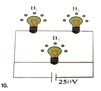
A 100 W bulb  $B_1$  and two 60 W bulbs  $B_2$  and  $B_3$ , are connected to a 250V source, as shown in the figure now  $W_1, W_2$  and  $W_3$  are the output powers of the bulbs  $B_1, B_2$  and  $B_3$ respectively then A.  $W_1 > W_2 = W_3$
