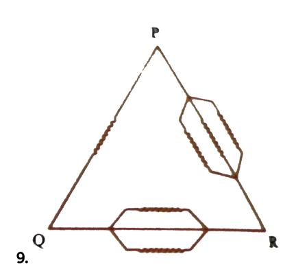
Six equal resistances are connected between points P, Q and R as shown in the figure. Then the net resistance will be maximum between
